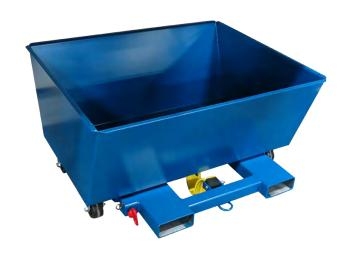
M.W. Watermark can provide a self-dumping cake hopper (also known as a dumpster) for almost any size press for easy handling of discharged solids. The hoppers are furnished with large ball-bearing casters for easy positioning under the presses, either manually or by using a lift truck. When filled, the operator picks up the hopper using a fork lift truck and positions it over a larger container. It's emptied quickly and easily by pulling the spring-loaded self-dump pin.
